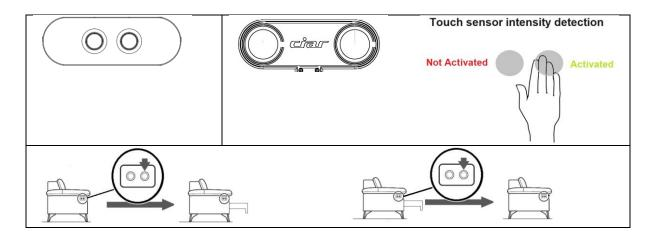
Extending the relax/sleep function - Hold down the button until the sliding mechanism extends and reaches the desired position and then release the button. The sliding mechanism will remain in the selected position.
